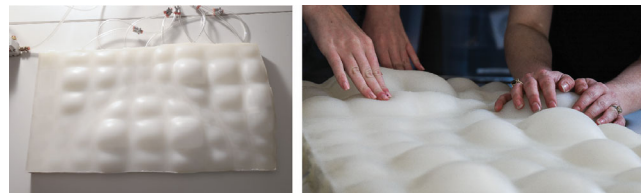
Figure 1. Soft Robotic Surface Panel (18 x 33 inches)
